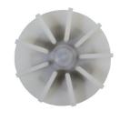
The combination of a solid metal core and a Fluopolymers lining (PFA \ PVDF \ PP) made by Transfer Moulding assures an excellent mechanical reliability and an optimal chemical resistance. The problem of reverse rotation during start-up has been eliminated thanks to the key driven system.
