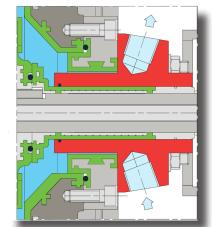
Same applications as conventional double seal Easy maintenance thanks to cartridge design
